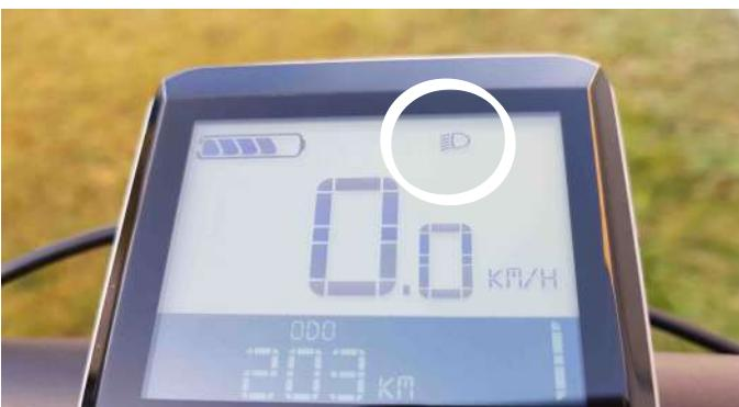
The speed release is obtained by pressing the Light button.
